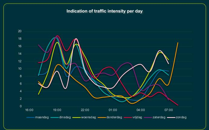
The traffic intensity is based on the number of triggers per hour, averaged over all sensors in the system.
